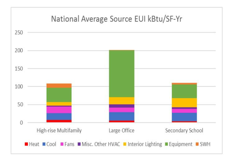
Based on PNNL Progress Indicator Models compliant with Standard 90.1 2013
